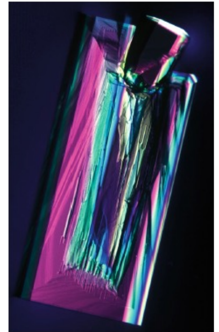
Rochelle salt under polarized light, showing evidence of different ferroelectric domains. Credit: Sciencephotos/Alamy Stock Photo
